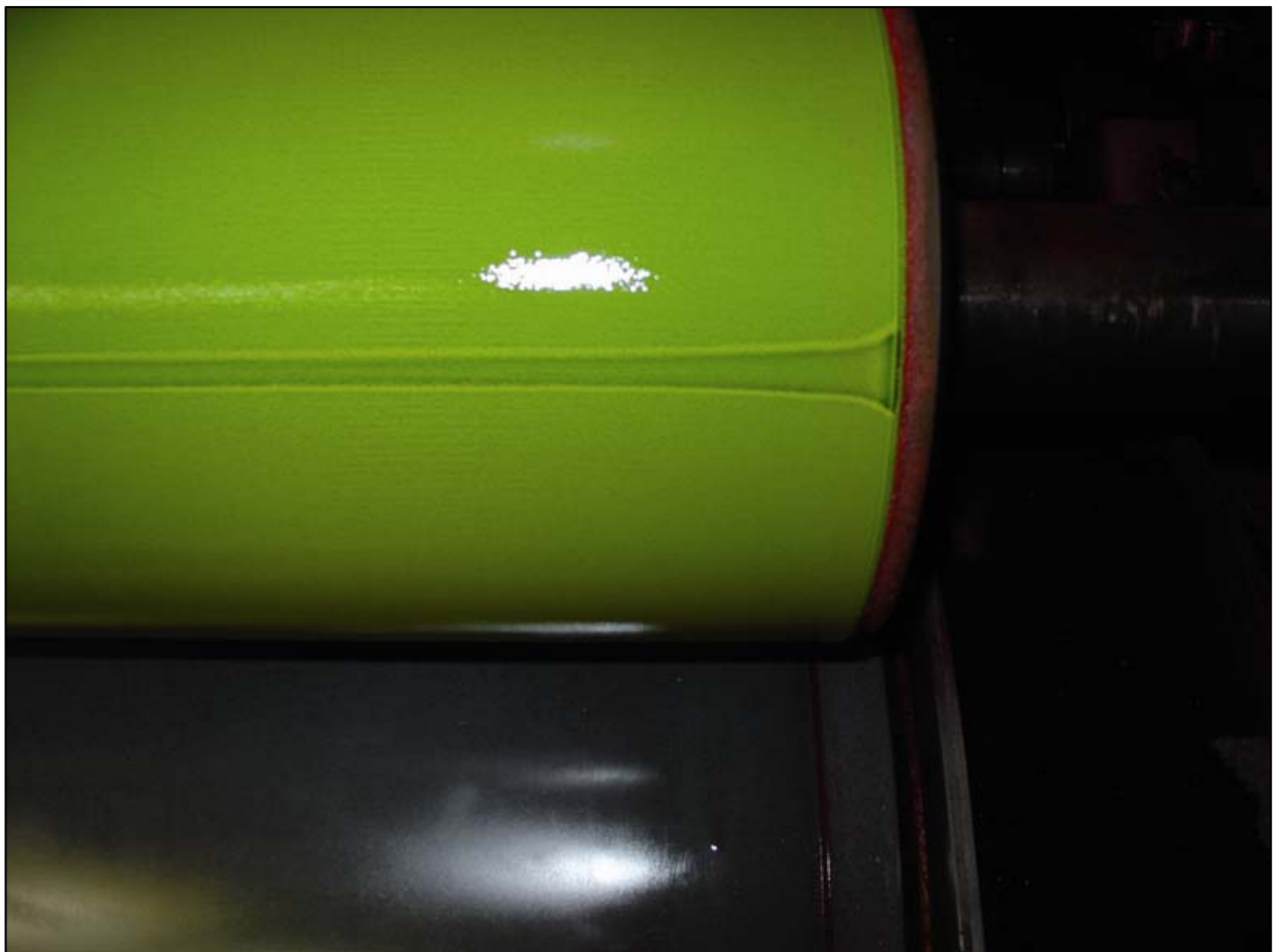
Fig. 4: Roller Stripe "Flaring" as a Result of Roller Shrinkage
