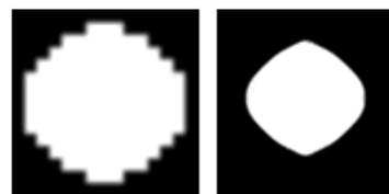
film output at "normal" imagesetter exposure (right) film output at "high" imagesetter exposure (left)
