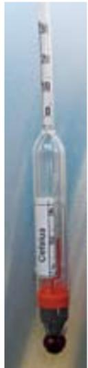
The areometer can be used to measure the IPA-content in the water. The device indicates percent by volume and by weight. Percent by volume should be principally measured. Since temperature plays an important role in determining IPA, please do pay careful attention to the temperature balance. Include the specific weight (density), of the dampening solution additive when making the determination (see the chart).
