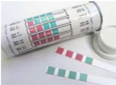
The overall hardness of the water may be measured simply by using test strips. Dip the hardness-strip briefly (1 second) into the water, then read the results after two minutes.
