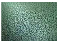
Cracking due to chemicals
