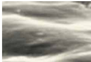
Glazed roller with calcification on the surface
