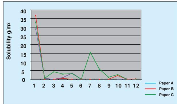
Adam's Wet Rub test of the three papers (A, B and C) with different fountain solutions. All three papers show a high solubility degree with fountain solution 1. Paper C is more sensitive for solubility of the coating than paper A and B.
