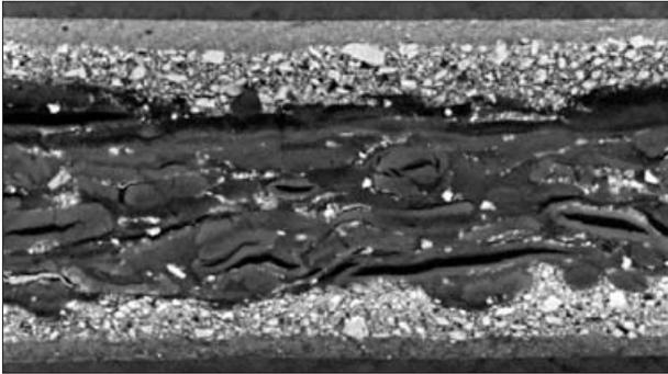
SEM-picture of a cross section of a coated paper. The lighter areas on top and bottom are the coating layers (double coated) and the dark area is the base paper
